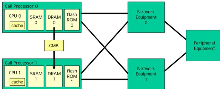
Larger M1 systems are shipped with dual Call Processor cards. Either CPU is powerful enough to drive the whole system, and each is connected to all peripherals. The backup CPU is held in reset state, and is not actually running. The inactive DRAM bank is kept in sync with the active one by the CMB ASIC.
